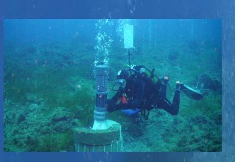
Scientific diver working on a submarine monitoring device for gas flow quantification close to Panarea, Italy (SDC TU Bergakademie Freiberg)
